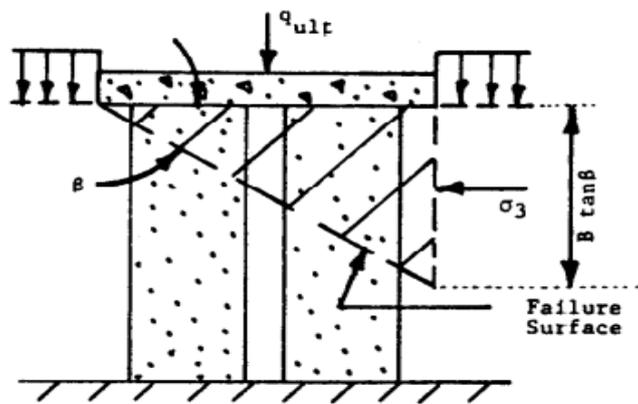
Figure 5. Failure mechanism of a group of DDC columns in cohesive soil .
