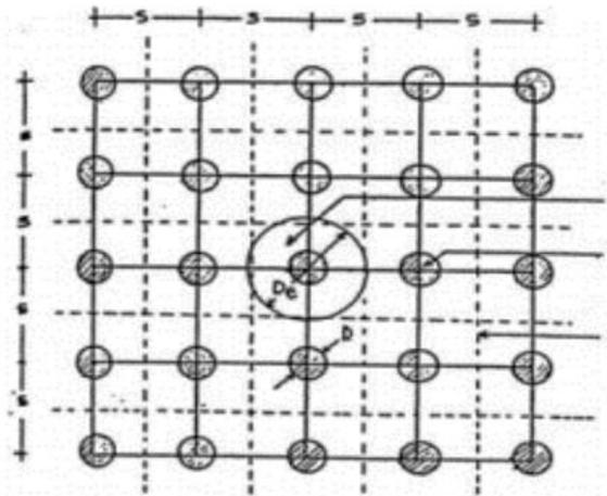
Figure 4. DDC Using Square Arrangement Pattern.
