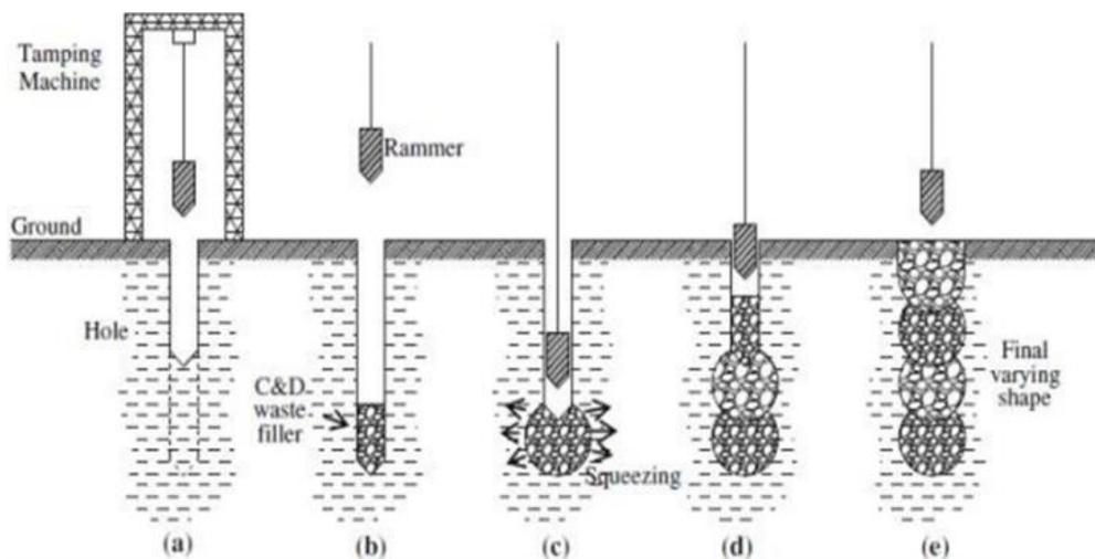
Figure 1. Self-tamping procedure
