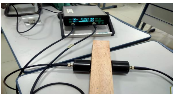
Figure 5. Ultrasonic Pulse Velocity Test
