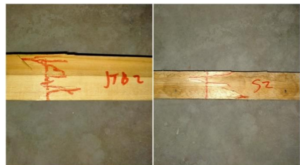
Figure 7. Damage patterns of jati (left) and sengon (right) woods
