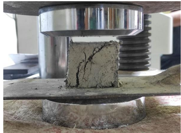
Figure 7. The test object after being compressed with UTM
