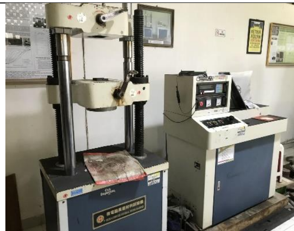
Figure 4. Universal Testing Machine (UTM) the Materials and Structures Laboratory, Civil Engineering Study Program UMY
