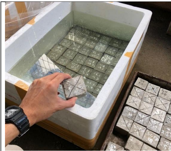
Figure 3. Curing cube test object of 5x5x5 cm 3
