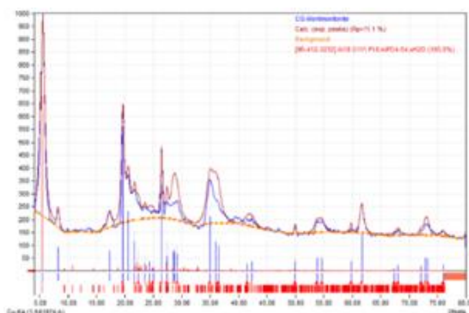
Figure 1. Diffractogram of montmorillonite powder
