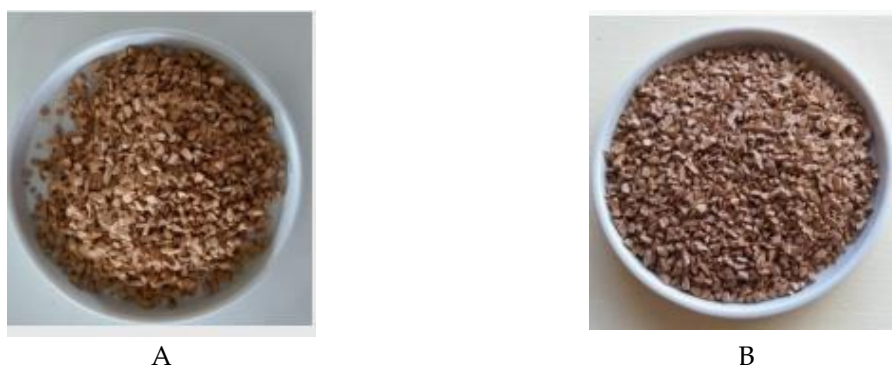
Figure 2. A. Montmorillonite granules; B. TiO 2 modified montmorillonite granule
