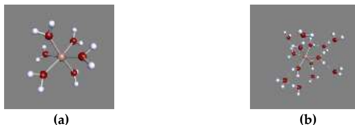
Figure 6. Snapshot of hydration structure of \text{In}^{3+} ion a) first hydration shell and b) first and second hydration shell
