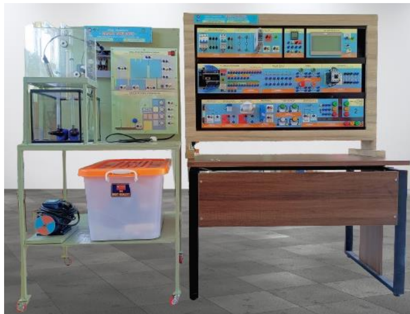
Figure 3. Smart Building Training Kit Product Equipped with SCADA Based on IIoT
