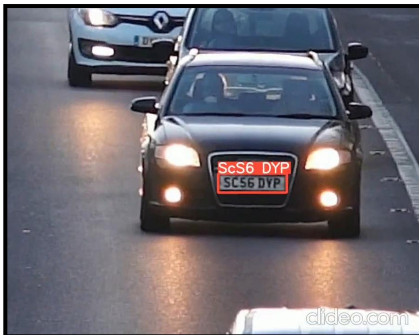
Figure 7. Result of Number Plate Detection System Reading with EasyOCR
