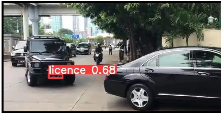
Figure 6. Result of Number Plate Detection System Reading without EasyOCR
