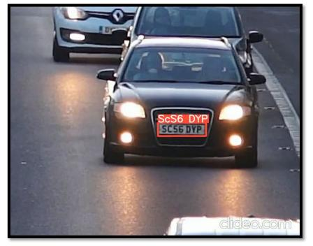
Figure 7. Result of Number Plate Detection System Reading with EasyOCR
