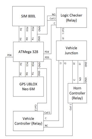
Figure 3. Circuit Block Diagram
