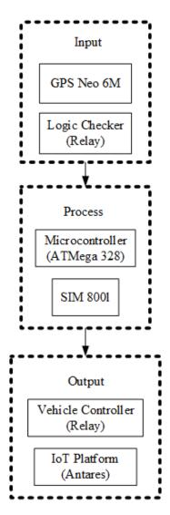
Figure 2. System Block Diagram
