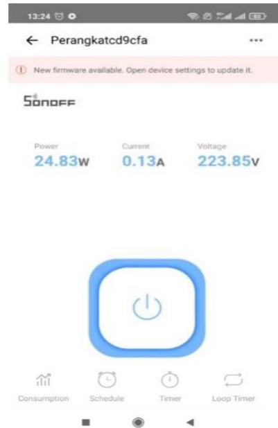
Figure 11. eWeLink display when Sonoff is connected load
