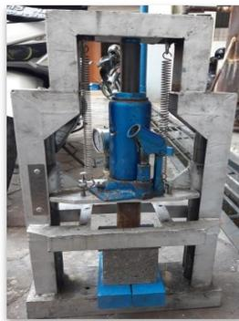
Figure 2. Briquette Compacting Device
