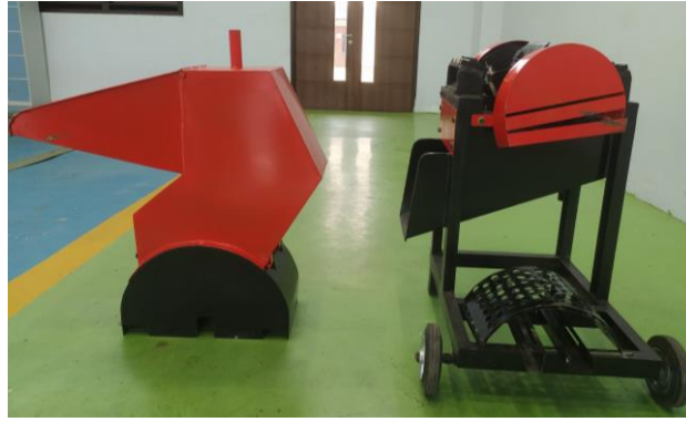
Figure 5. Results of Plastic Shredding Machine Manufacturing HSS Crusher Type
