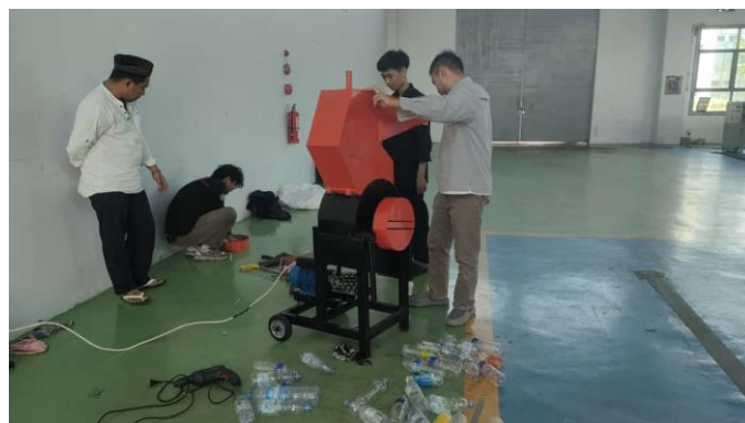
Figure 6. Performance Trial Process of Plastic Shredding Machine HSS Crusher Type
