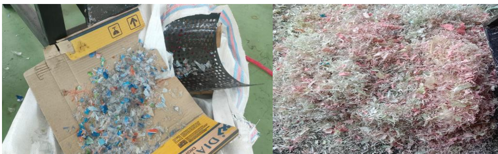
Figure 7. Results of Shredding Plastic Bottles Plastic with Shredding Machine HSS Crusher Type
