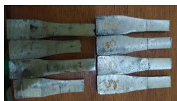
Figure 3. Specimen for tensile test.
