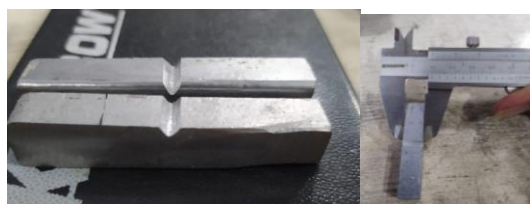
Figure 6. Specimen for punch test.
