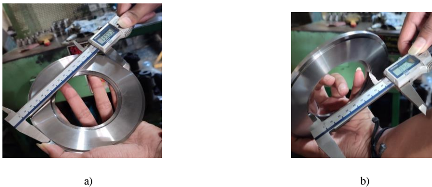
Figure. 4 OP1 production results front section of a) Outer diameter and b) Inner diamter on a CNC lathe.
