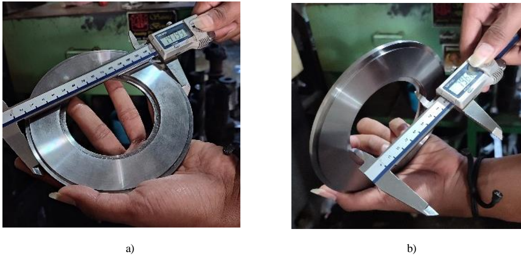
Figure. 5 OP2 production results rear section of a) Outer diameter and b) Inner diameter on a CNC lathe.
