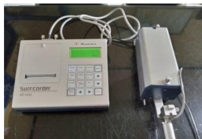
Figure 2 Measuring Instrument Surface Roughness Tester TR 1200
