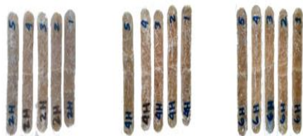
Gambar 4. Sample uji impact
