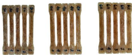
Gambar 3. Sample uji tarik
