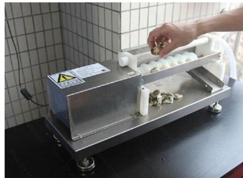
Gambar 5. Alat Pengupas Kulit Telur Otomatis (Sumber: Aliexpress, 2021)
